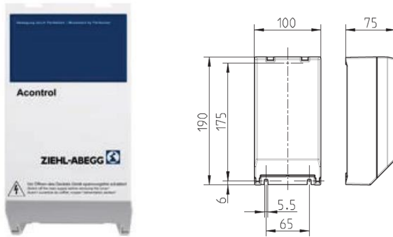
Figure 16: PKE-6 Fan speed controller details and dimensions
